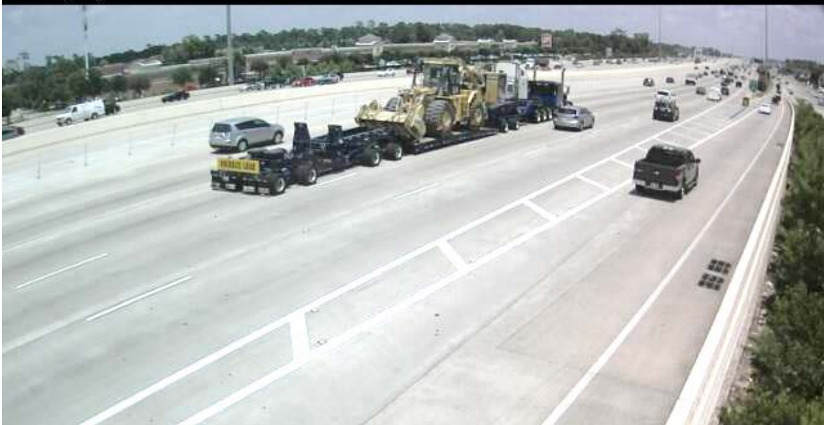
Figure 10. Designated Oversize Load Detected as Overheight at the Wirt Site.
